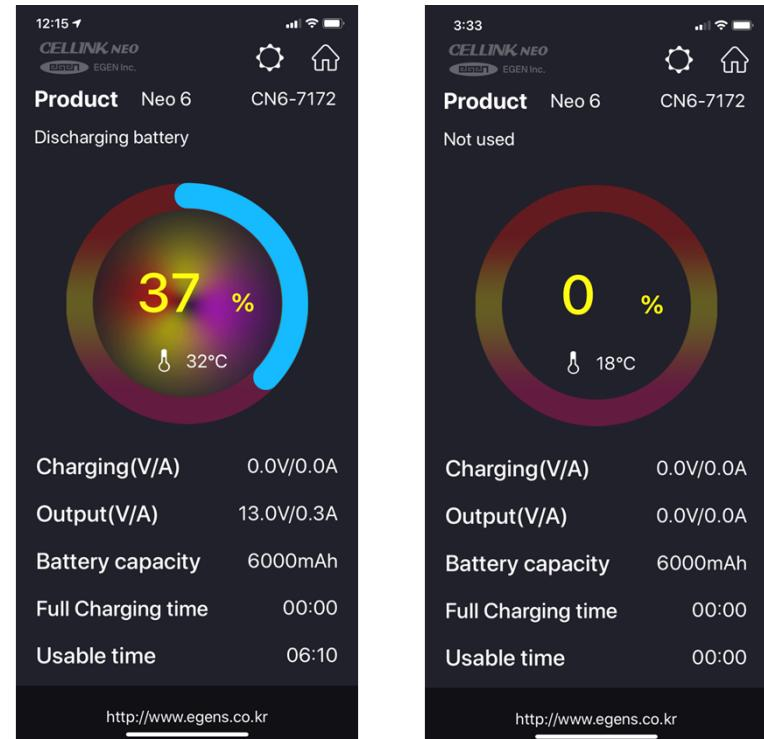
Screen shot of Cellink Neo6 battery discharging while parked (6hr 10 min to go), and fully discharged overnight. F273 takes approx. 7 mins to shut down after ignition off, whereas a Power Magic Pro will continue to discharge the car battery until it hits the voltage settings set by the user.
