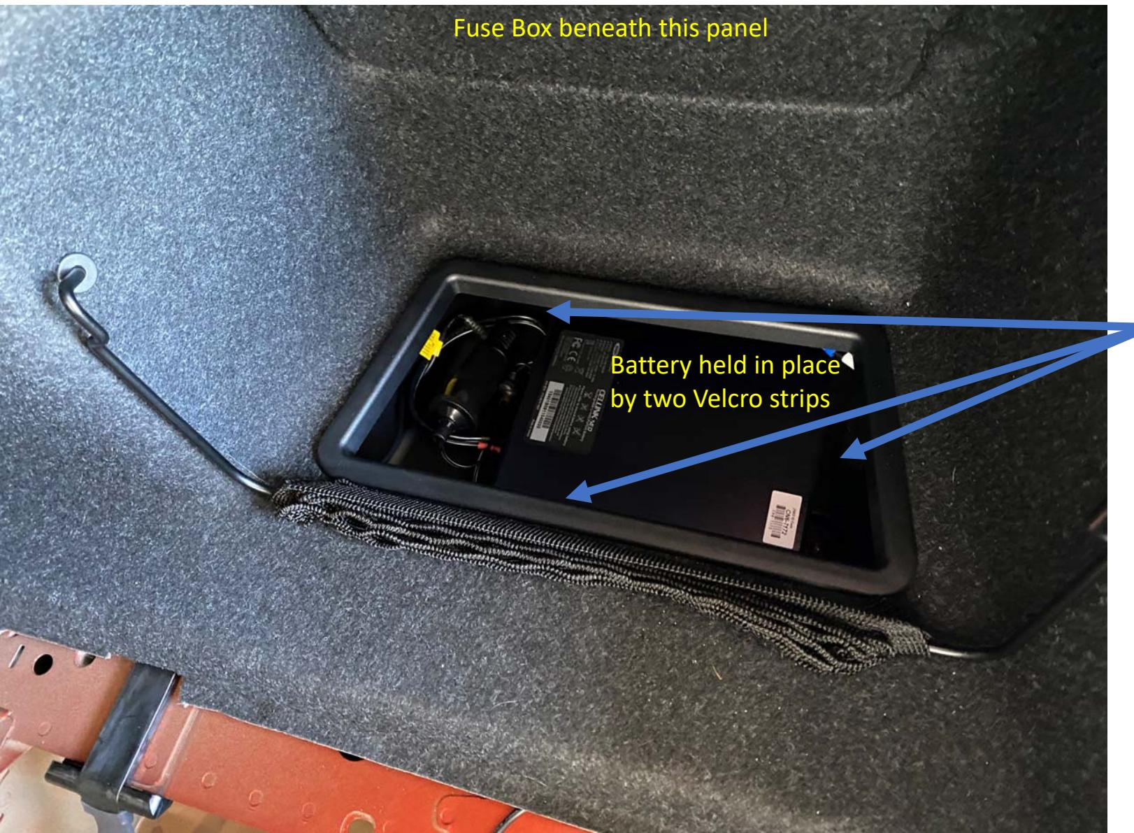
There is a small gap between the tray which is bolted to the floor and the rectangular plastic that normally holds the first aid kit.
